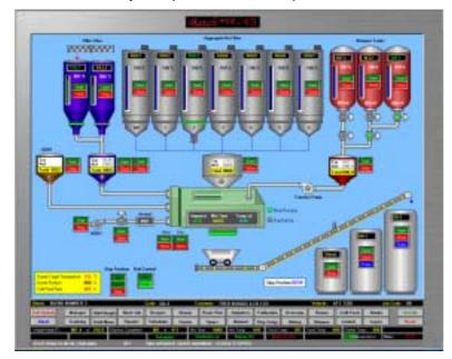
system. As a companion product of which controls operations only **Batch**<sup>+ve</sup> takes care of everything from cold feed to hot storage. Plant operation automatically controlled by the latest Mitsubishi Q series PLC and a Windows based SCADA and graphics system designed by ATS. New features include redesigned graphics and a completely new recipe editor and job scheduling combination which together with the updated expanded reporting facilities makes this one the product to beat.
